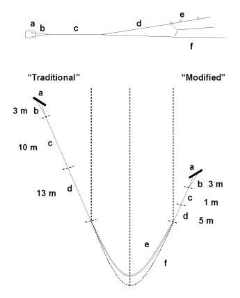
**Figure 3.** Diagram of traditional and modified designs used in the experimental fishing. a: Otter boards, b: Door legs, c: Sweep, d: Bridles, e: Headline, f: Footrope.
