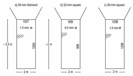
**Figure 2.** Diagrammatic representation of a) the control 26 mm diamond-shaped mesh polyamide-PA codend, b) the 32 mm square-mesh (22.5 mm outside bar) polyethylene-PE codend, and c) the 30 mm square-mesh (16 mm outside bar) polyamide-PA codend used in the experiment (T: transversals, B: bars, N: normals).
