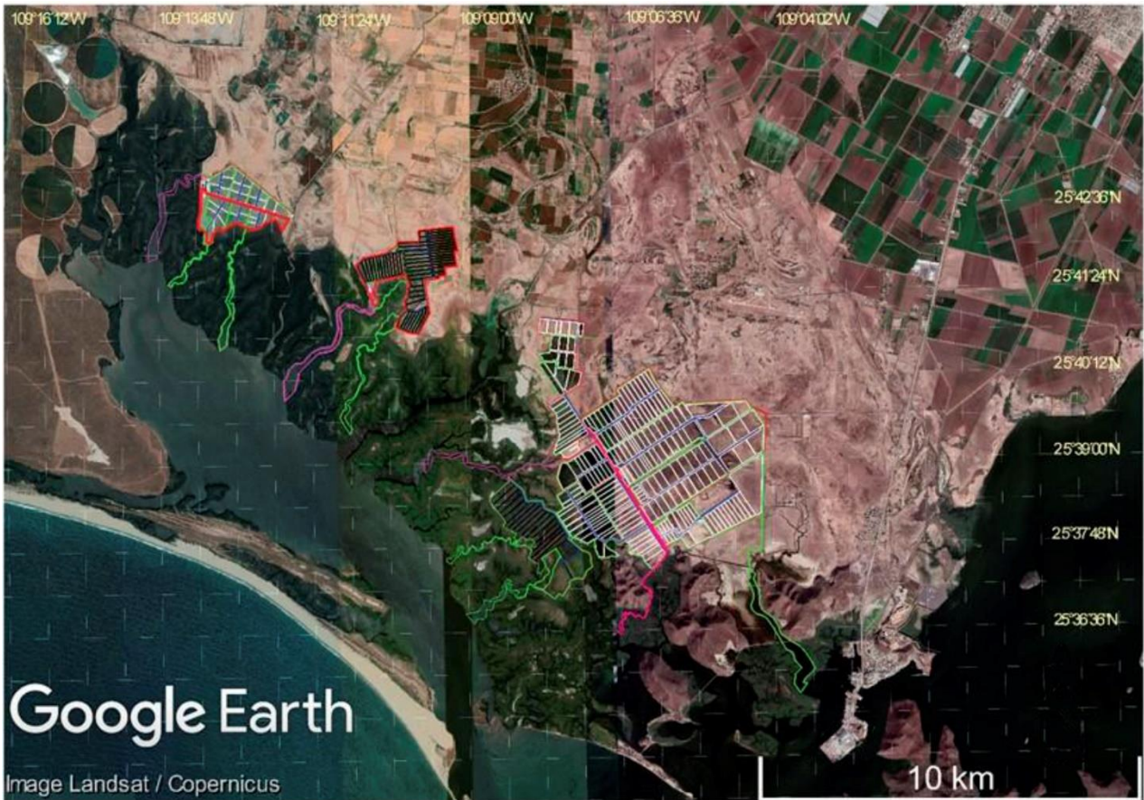
Figure 5. Shrimp production infrastructure includes intake canals (magenta), discharge/harvesting canals (green), and grow-out ponds. These components play crucial roles in regulating water flow, maintaining water quality, and providing controlled environments for shrimp rearing. Understanding their spatial arrangement and functionality is essential for effective shrimp farming and system management.
