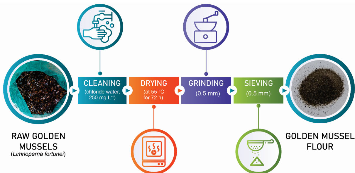
Figure 1. Flowchart summarizing the steps of whole mussel flour preparation. Source: author's archive.
